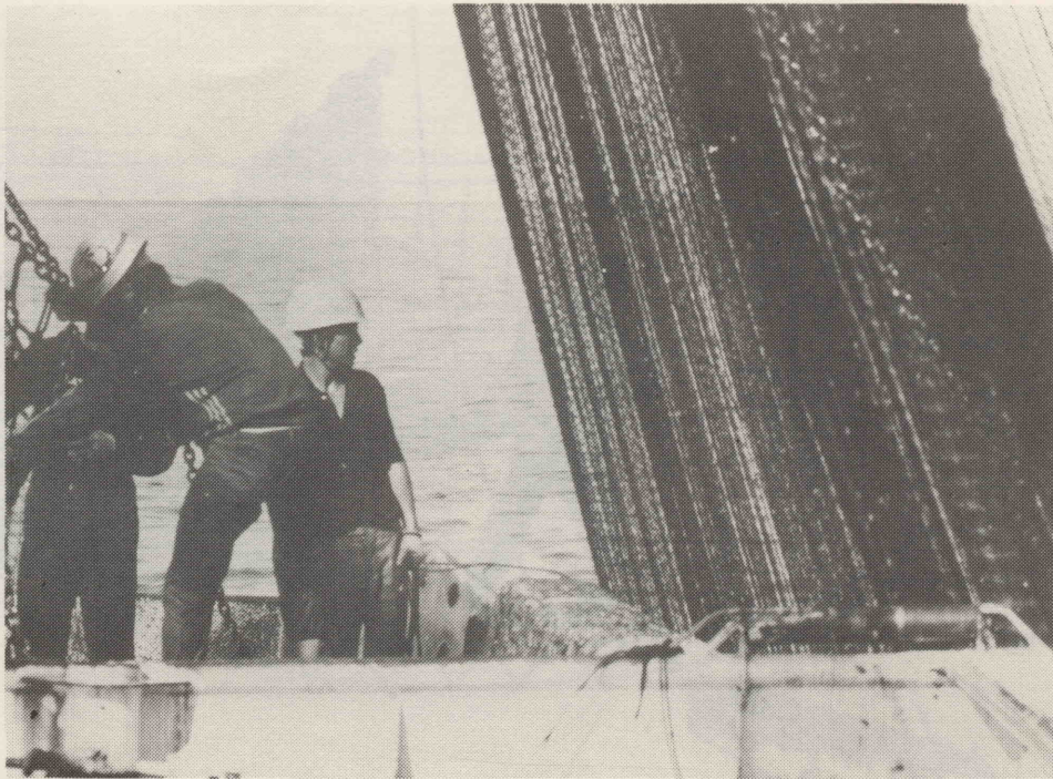
The net is hauled on board and carefully laid out ready for the next school. The net is folded to the left of this photograph but the sinker chain can just be seen here on the left and the purse-ring chains are laid out in the middle of the photograph
