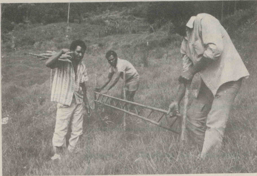
Using the landlevel to make out a contour line Photo: J. Wankowski
