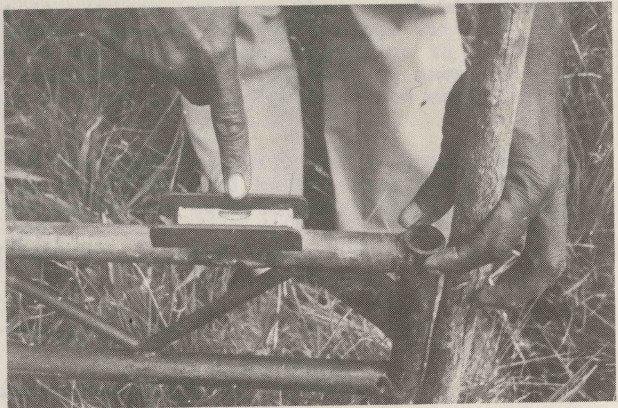
Checking that the bubble is centred properly Photo: J. Wankowski
