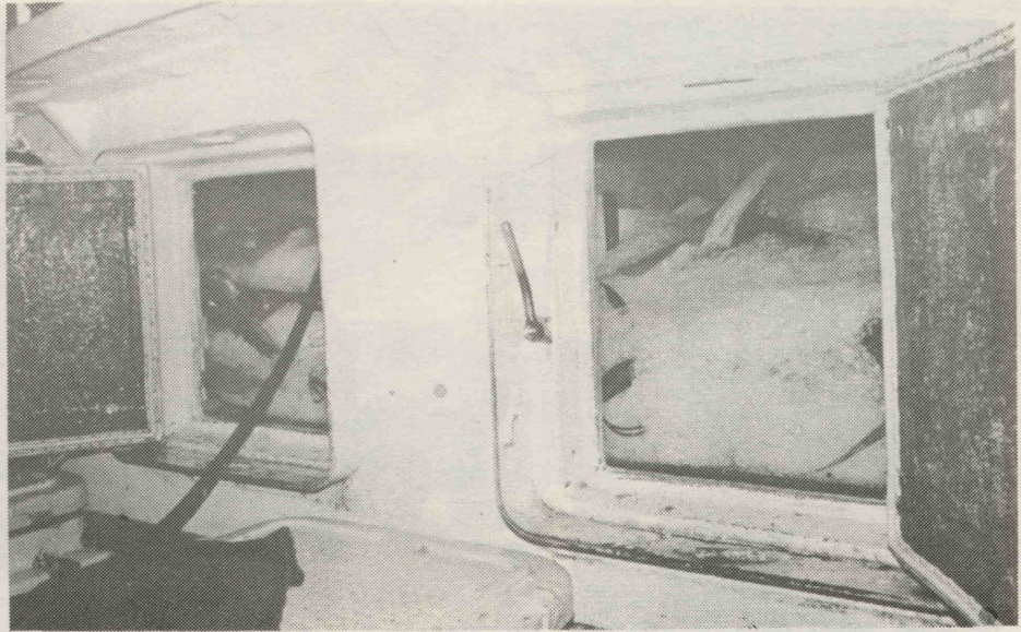
About three tonnes of the catch for the whole voyage is put on flake ice. The rest of the fish are kept in sea-water chilled to between -0.5 and -0.7^{\circ}\text{C} .
