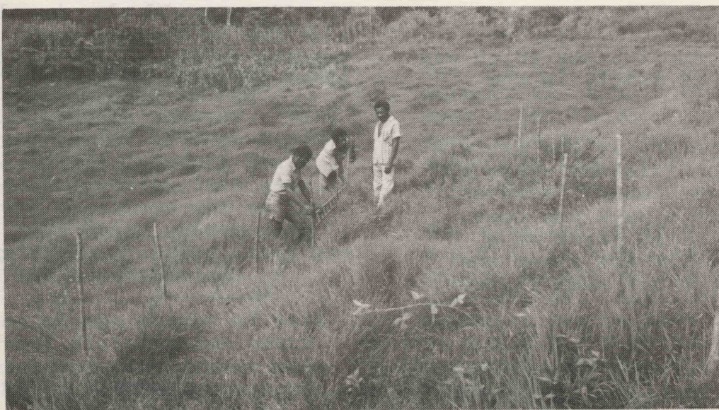
Using the land-level to mark out contour lines in the field Photo: J.W.J. Wankowski
