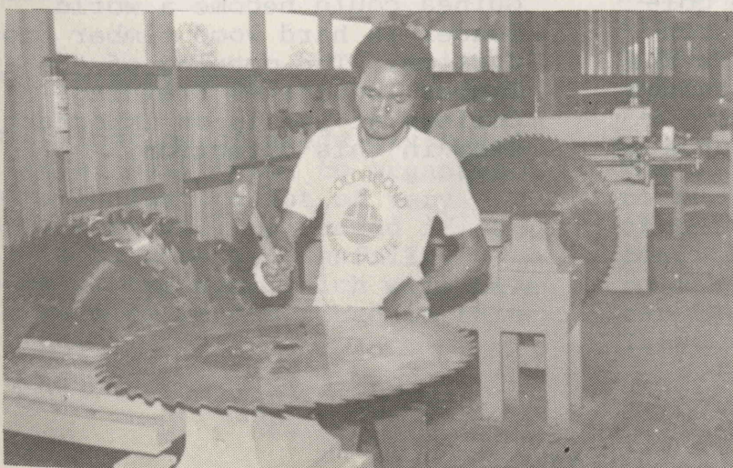
To tension a saw, the student beats it very carefully with a heavy hammer.
