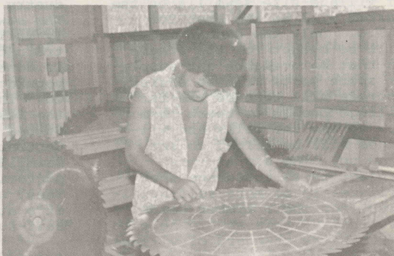
The student in this picture is chalking up a saw ready for tensioning.
