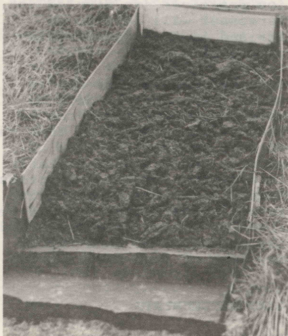
A 2 m 2 microplot on a 10 degree slope, used to measure soil loss due to rain-splash and slopewash erosion. Half a 44 gallon drum is used as a collection tray at the lower end of the plot.
