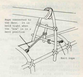
Detail of the door of the trap, to show how the ropes are attached
