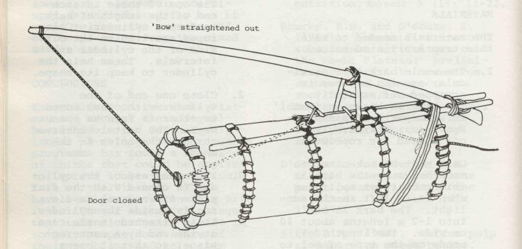
The construction and operation of the eel trap. In the top diagram, the door of the trap is held open by ropes which connect the door to the 'key knob' and to the 'bow'. In the lower diagram, the bait has been pulled down. This loosens the horizontal bar (A), and so releases the vertical bar (B) in the 'key knob' This then allows the 'bow' to spring back to a straight position. At the same time the door is pulled closed.
