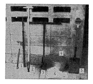
take more accurate samples at different depths, as well as surface samples, using a soil auger or a soil sampling tube.
