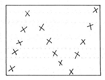
The correct method of taking samples. Each x represents a sample
