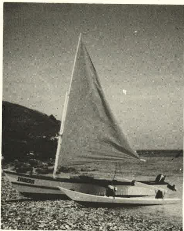
The Red Snapper canoe "Iamera" was the first of these canoes to be completed. Side (left) and front (right) views, showing the gunter rig sail.
