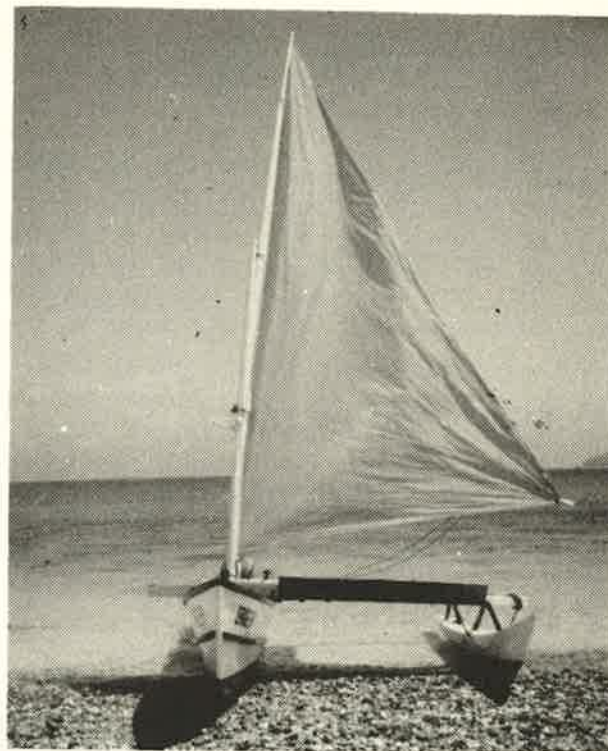
The Red Snapper canoe "Iamera" was the first of these canoes to be completed. Side (left) and front (right) views, showing the gunter rig sail.
