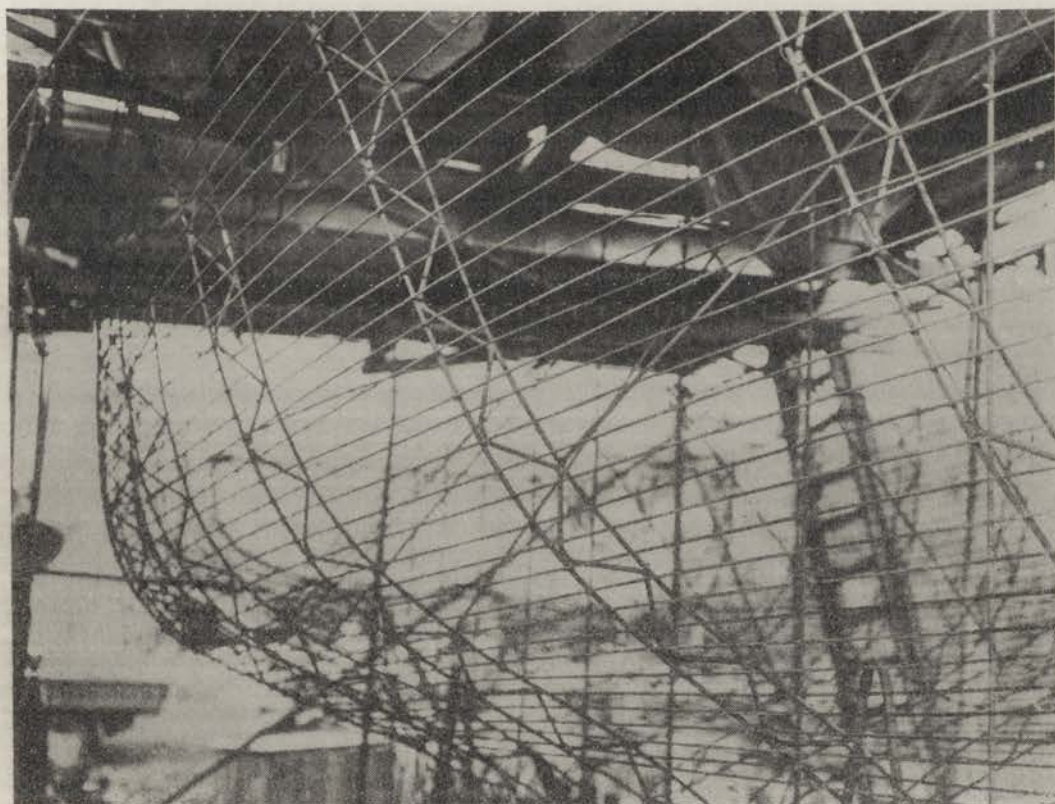
Plate II. —Frames, stringers and vertical suspenders
