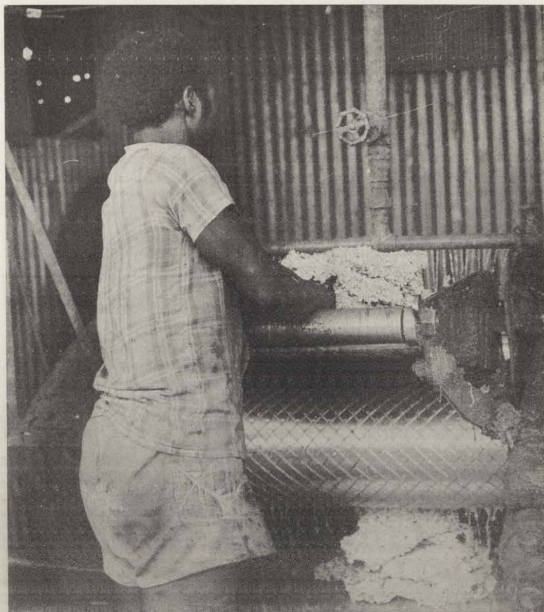
Plate I.—Ground scrap being processed. The rollers have a tearing action and foreign material is washed out of the rubber.
