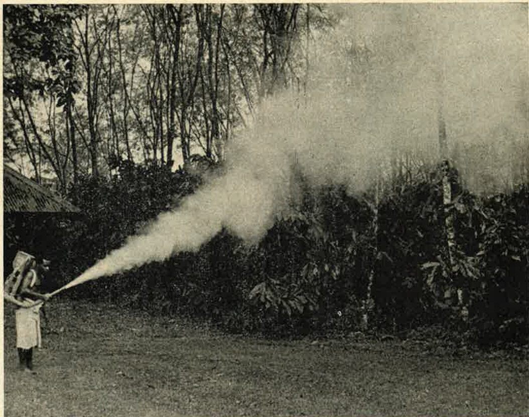
Plate III.—A shoulder-mounted motor-driven duster in action.
