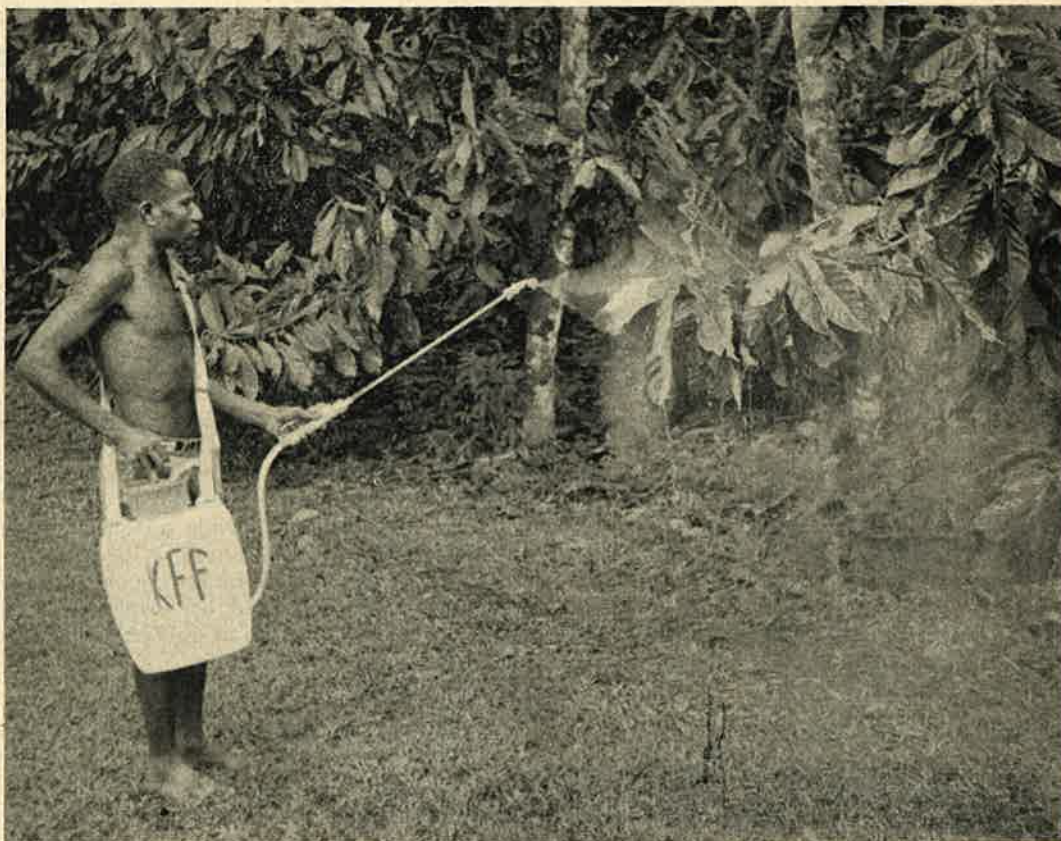
Plate I.—A type of hand-operated knapsack sprayer used for high volume application of chemicals.—N.B.—Excess spray running off.
