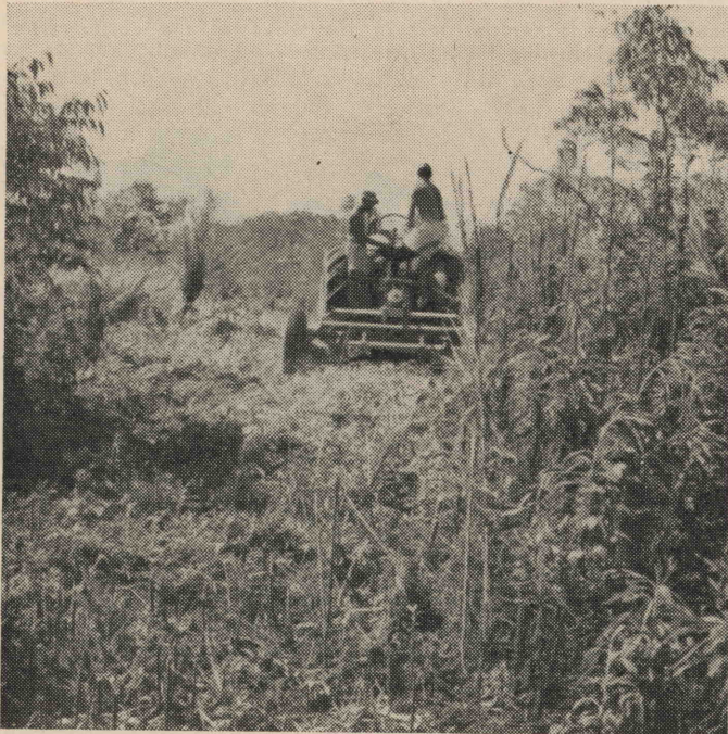
View of the cutter at work in secondary growth being drawn by 30 h.p. International AW.6 tractor.
