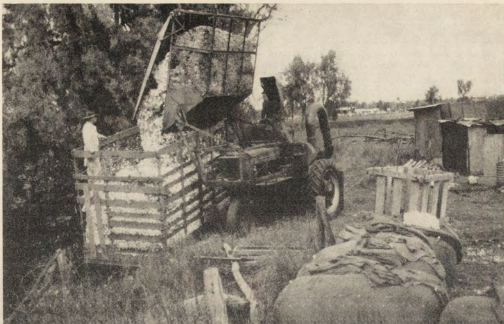
Plate VIII.—Unloading directly from the harvester to a farm truck. (The harvester bin holds 700-800 lb. Bales of cotton in right foreground.)
