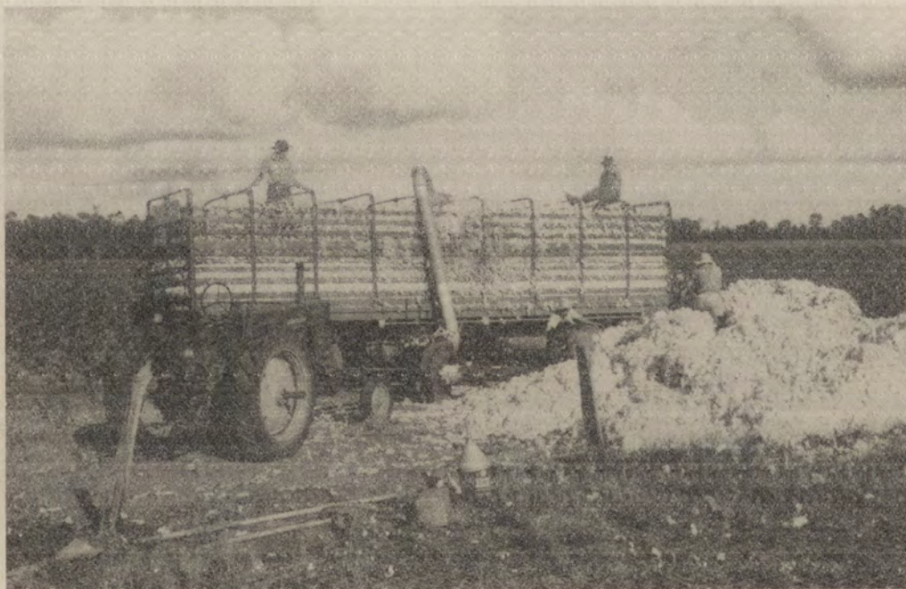
Plate IX.—Cotton being loaded onto a semi-trailer by a portable blower.
