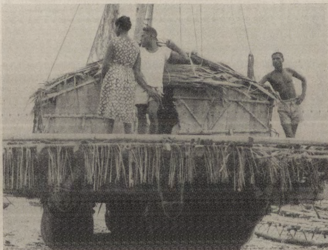
Plate III.—Three-hulled canoe showing hulls and deck house.
