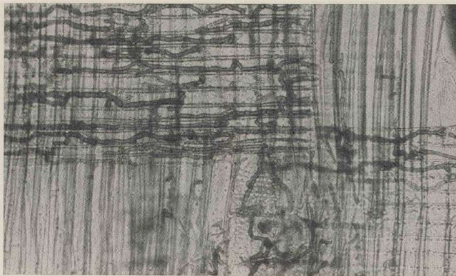
Plate V.—Section through "blue stain" area of damaged Leucaena , showing strongly orientated brown hyphae in the parenchyma but relatively few hyphae in fibres and xylem. \times 250 .
